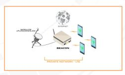
Beacon's Emergency Response Cellular (ERC) can be deployed rapidly to re-establish connectivity within minutes through a Private LTE Network. Worldwide communication (via the Internet) can be established through a mobile satellite link or dark fiber interconnectability.
